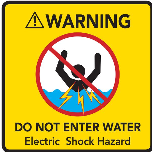
Any docked boat while plugged into shore power is an electric risk. Without ELCI protection, electric current can inadvertently leak into waters. This leakage is typically due to faulty wiring in the boat's equipment or the dock's shore power. Anyone nearby in the water could suffer from paralysis or electrocution (a phenomena called Electric Shock Drowning, or ESD).
